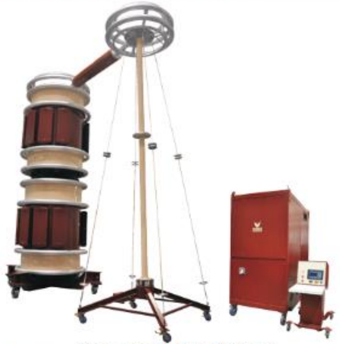
AC, Cascade Type, 400 kV, 800 kVA
